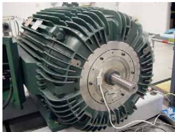
Figure 4. Industrial motor supported on magnetic bearings with integrated electronics.
