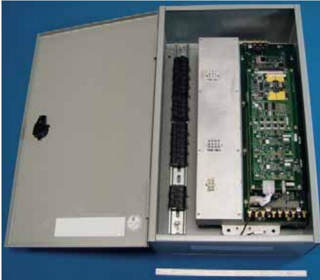
Figure 5. Compact magnetic bearing controller
