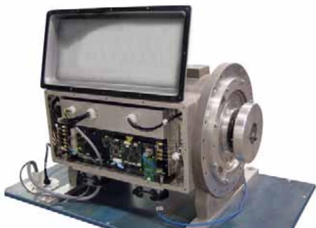
Figure 2. High speed drive train on magnetic bearings. Motor shown is 400-kW at 20,000-rpm.
